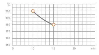
Please observe cure parameters closely since mechanical properties will develop before full cross-linking!
